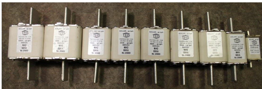
Photo 2: Fuses after all tests, rating plates
